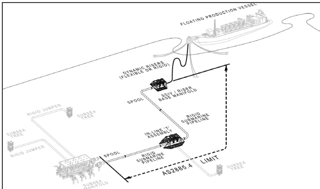
**Figure 2 – Application Limits between Subsea and Floating Facility**
