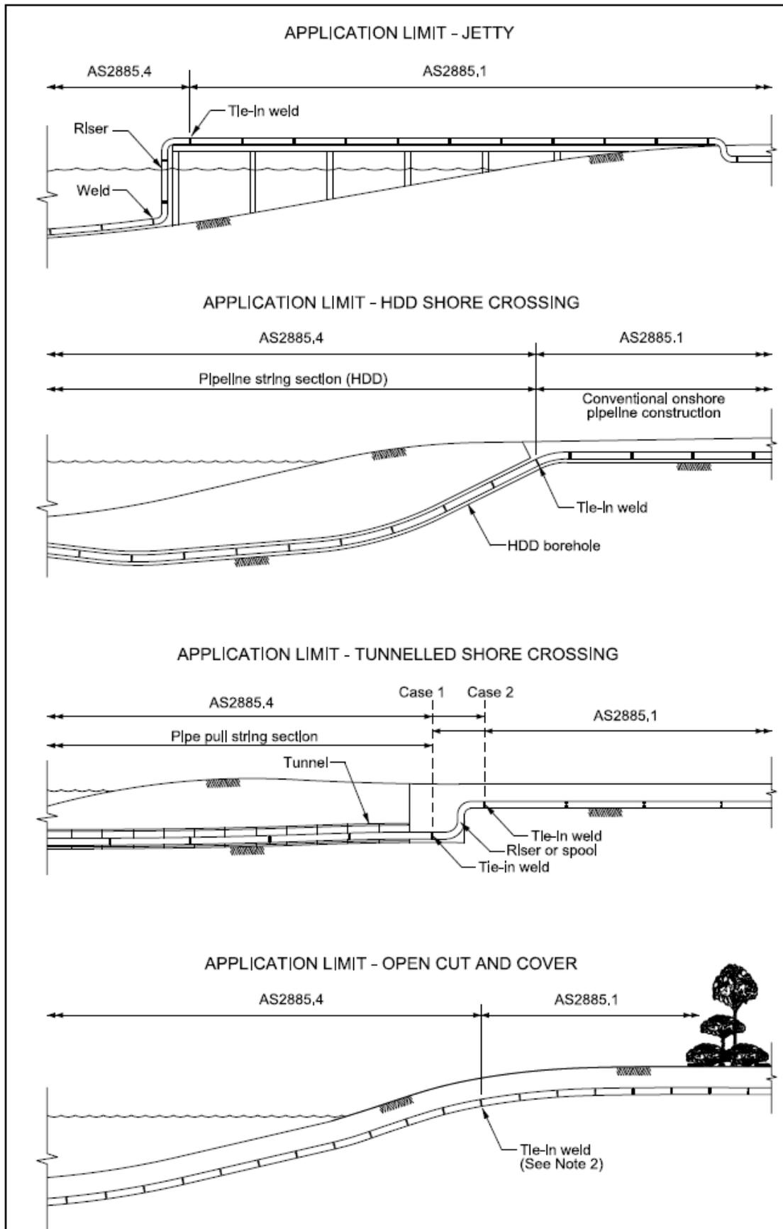
Figure 3 – New Code Break Locations between AS/NZS 2885.1 and AS/NZS 2885.4
