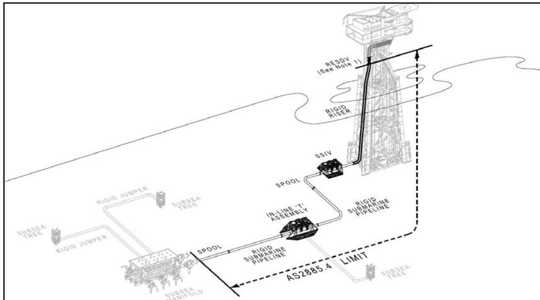
**Figure 1 – Application Limits between Subsea and Fixed Facility**
