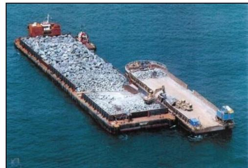
Figure 2 – Side Dump Vessel with Engineered Rock
