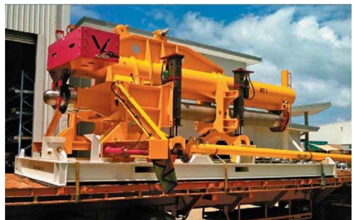
Figure 4: Sleeper with Imposed Lateral Displacement
