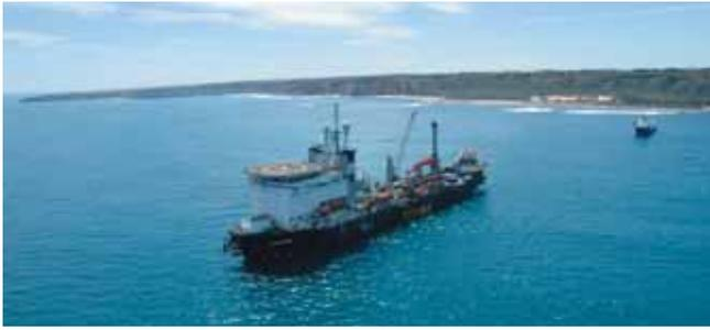
Figure 5. A laybarge recovering the pre-installed pipeline string at an HDD site.
