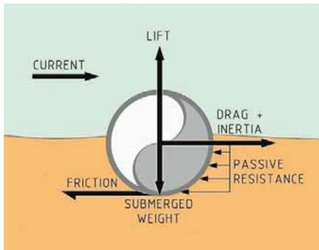
Figure 1. Force model of subsea pipeline stability.
