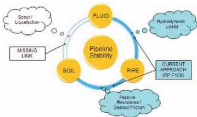
Figure 3. The missing link in the current approach.
