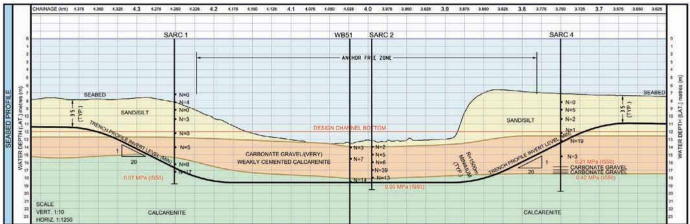
Figure 3. A section of the shipping channel crossing.
