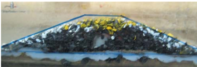
FIGURE 5 : BERM PROFILE AFTER 1,000 YEAR RP TEST
