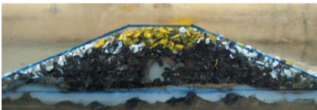
FIGURE 4: BERM PROFILE AFTER 100 YEAR RP TEST
