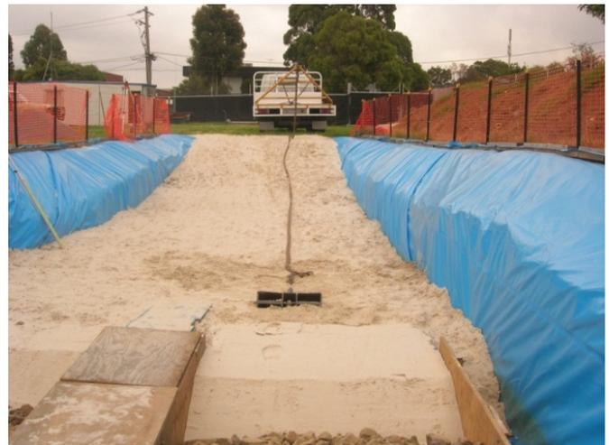
FIGURE 5: ANCHOR DRAG MODEL TESTING
