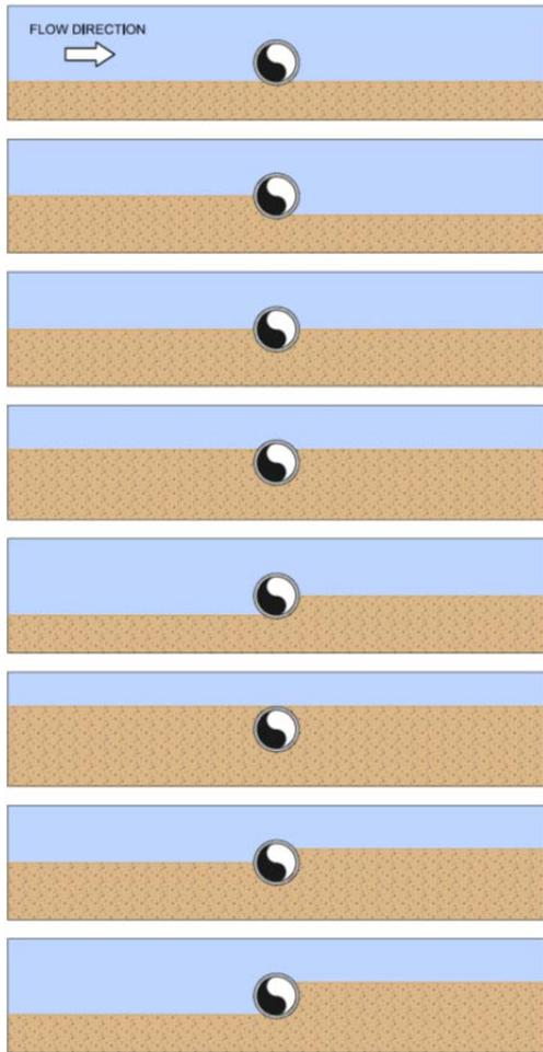
Figure 7: Initial Embedment Profiles Tested in O-Tube
