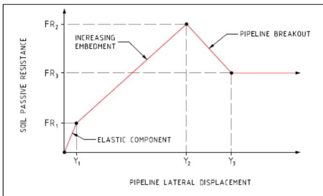
Figure 11: Verley Force-Displacement Curve (Ref. 3)
