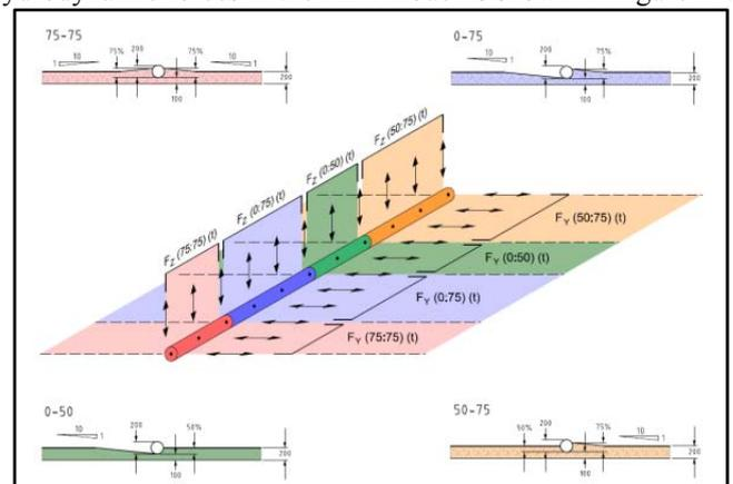
Figure 14: Application of Hydrodynamic Loads in FEA
